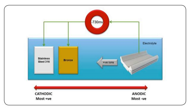
All metal generate voltage in water. The metal gives up electrons resulting in positively charged ions, thus leaving electrons which give the metal a negative charge. The more negative the voltage, the more active the metal and therefore the higher the rate of corrosion.
