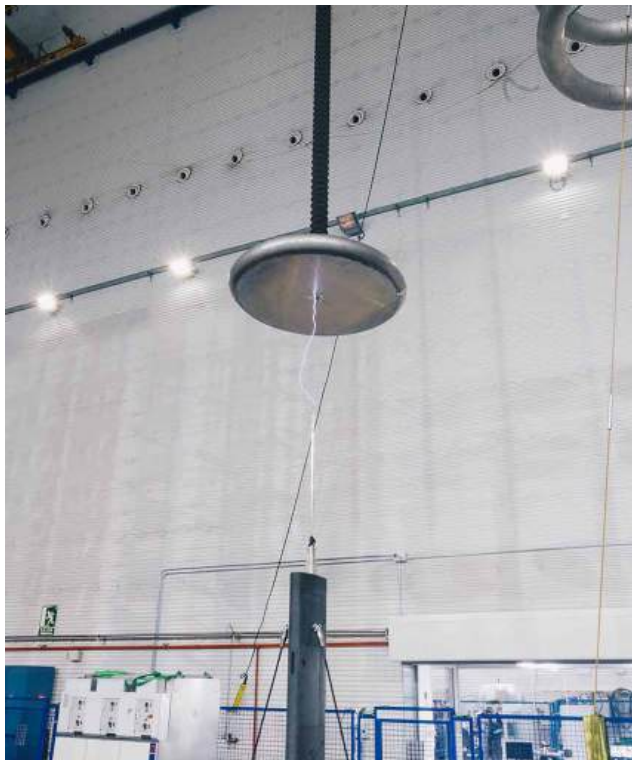
Southern Spars, Future Fibres, and RigPro launched an R&D project where over 350 lightning strikes were replicated.
